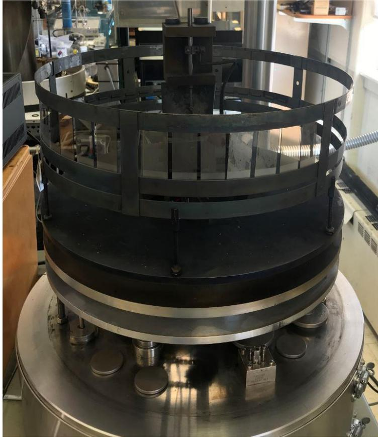
Figure 1: NRC Evaporator dedicated to carbon foil production
