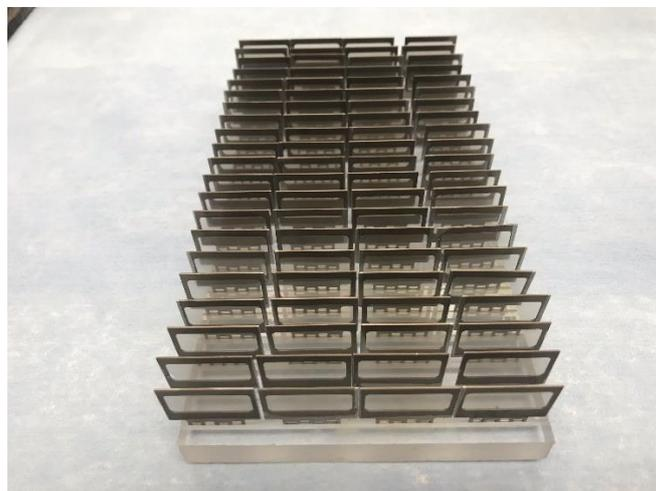
Figure 2: LPA foils mounted on frames ready for installation
