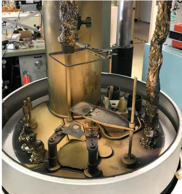
Figure 3: Veeco evaporator with e-gun and resistive heater
