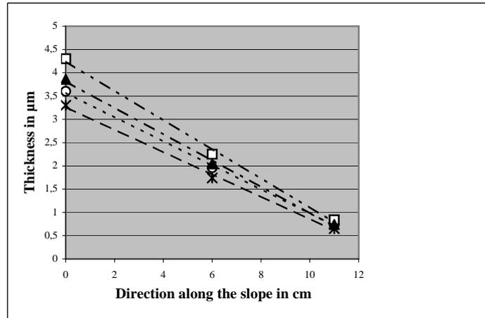
**Figure 2:** Measured thickness and linear fit for four Al-foils with different thickness gradients.
