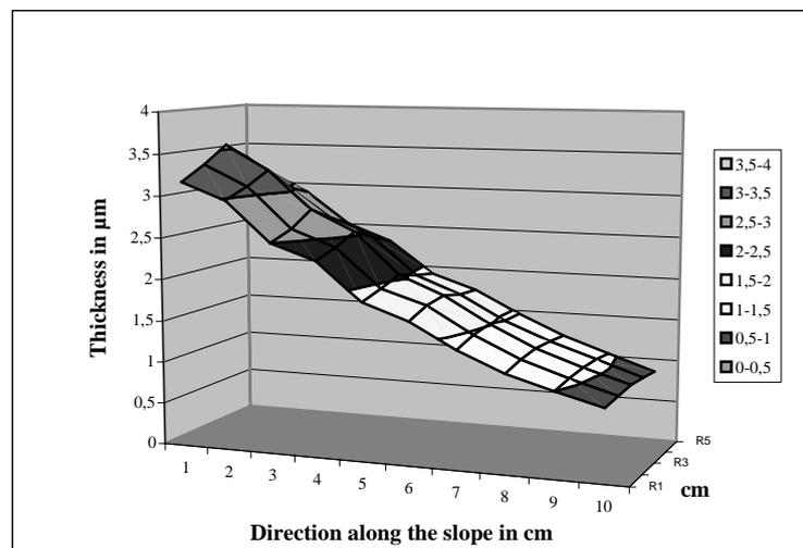
**Figure 1:** Thickness distribution of one aluminum foil determined by weighing the cut parts with 1 cm<sup>2</sup> area each.
