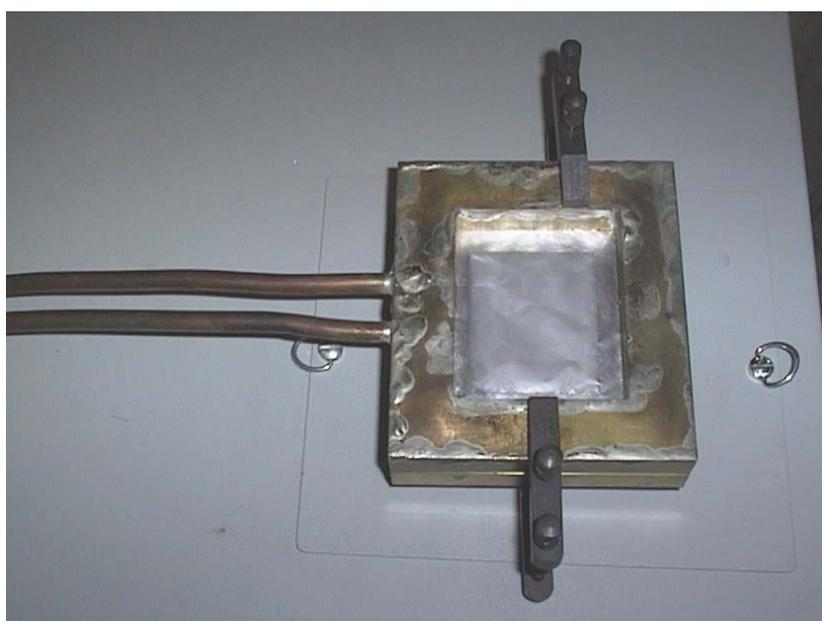
Fig. 2. The cooling jig used to protect the glue used for the target mounting
