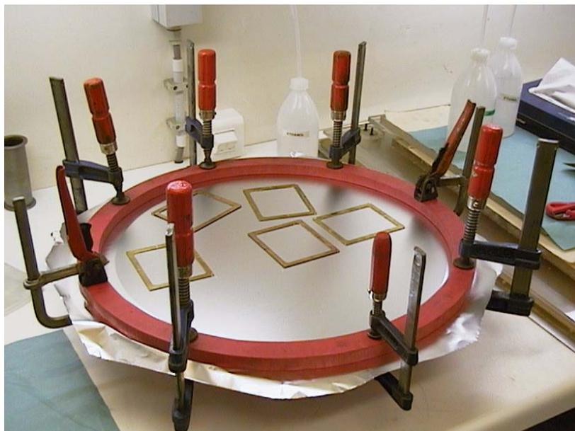
Fig 1. Foil tensioning jig with target frames glued in position
