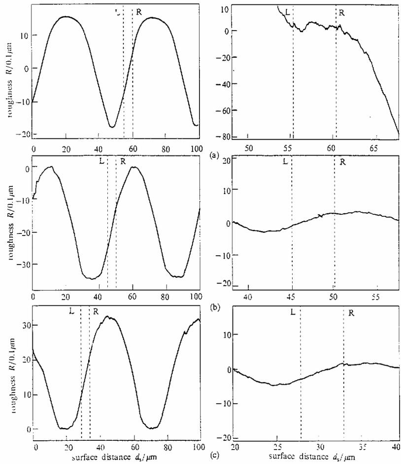
Fig. 3. Surface roughness on surface perturbation target of Brominated polystyrene
