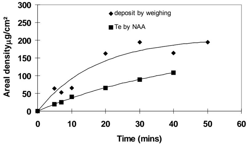
Fig. 3. Increase of target areal density (by weighing) and Te (by NAA) after deposition times up to 50 mins. Current density  $5\text{mA}/\text{cm}^2$
